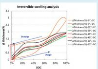
No matter the temperature rises from room temperature (25°C) up to 45°C and 60°C, or drops to 0°C, the irreversible swelling of the cell increases. However, the causes of irreversible swelling may be different under high temperature and low temperature conditions
