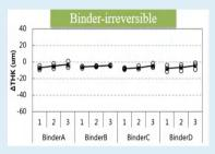
Comparison of the swelling behaviors of four LIBs made by different binders, the level of irreversible swelling is the same, and the main difference lies in the single-cycle swelling thickness,
