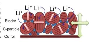
or other more serious consequences, such as the deformation of the LIBs, the fragmentation of material particles, the rupture of the solid electrolyte interphase(SEI), and the consumption of electrolyte. Thus, the swelling behavior of the LIB becoms an impotant indicator for evaluating the reliability of the battery. During the production process, the particle size, binder and must be optimized in advance.
