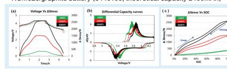
In the range of 5000N, with the increase of the pre-load, the swelling stress of the cell increases gradually, which leads to the increase of the polarization of the cell and the deterioration of the dynamic performance. Therefore, we must pay attention to the influence of the initial pressure When designing cell packing.
